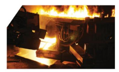
MTAG Switzerland's Robotemp is mounted on the floor next to the EAF so that both measurements and samples can be taken through the furnace door without changes to the EAF and so cartridges can be exchanged in the safe parking positions.
